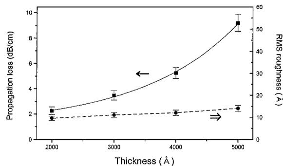
Figure 5. Propagation losses and RMS surface roughness of PLT28 films on MgO substrates as a function of film thickness.
