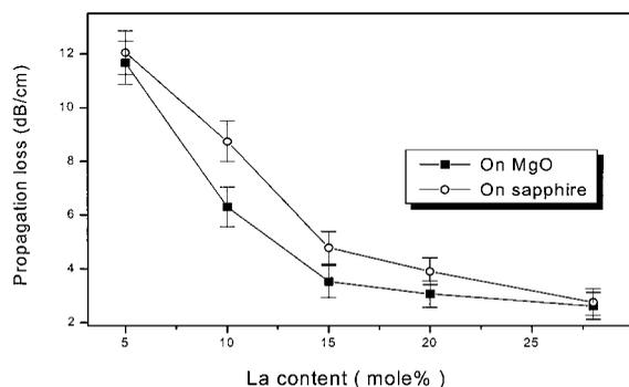
Figure 3. Propagation losses of PLT films fabricated on MgO and sapphire substrates as a function of La content.
