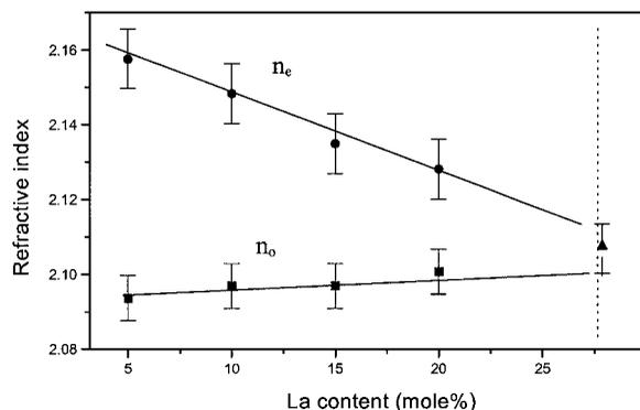
Figure 2. Refractive indices  $n_e$  and  $n_o$  of PLT films on MgO substrates as a function of La content.
