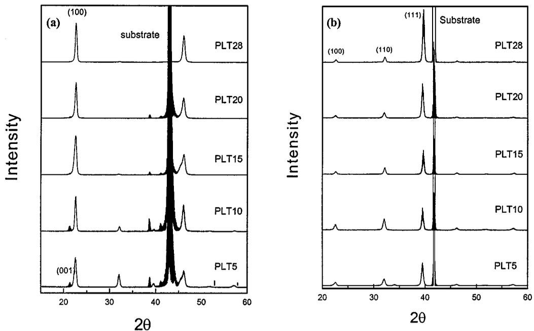
Figure 1. XRD patterns of PLT films on (a) MgO(100) substrates and (b) *c*-plane sapphire substrates as a function of La content.
