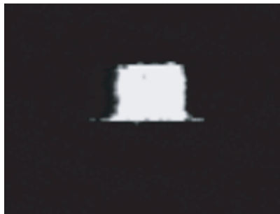
Fig. 8. Output near-field pattern of multimode waveguides.
